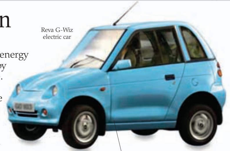
The G-Wiz has a range of 40 miles (64 km) and a top speed of about 40 mph (64 kph)
