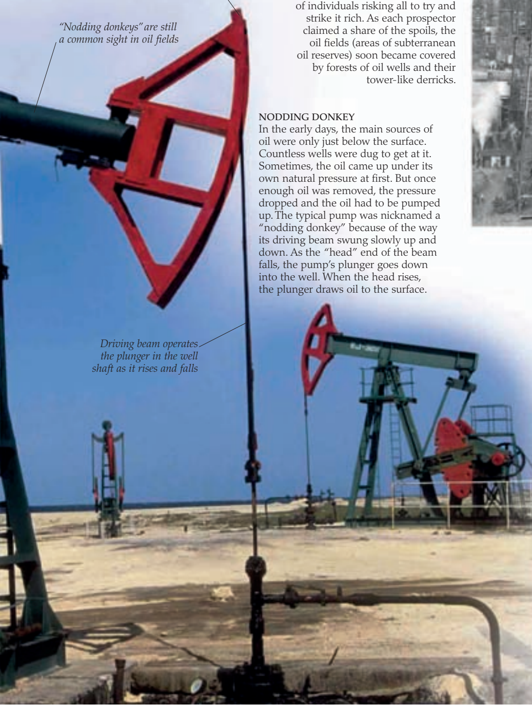
The curved end of the beam is likened to a horse's head in the US.
