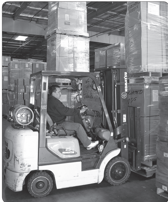
Natural gas is used to power some fork lifts.
