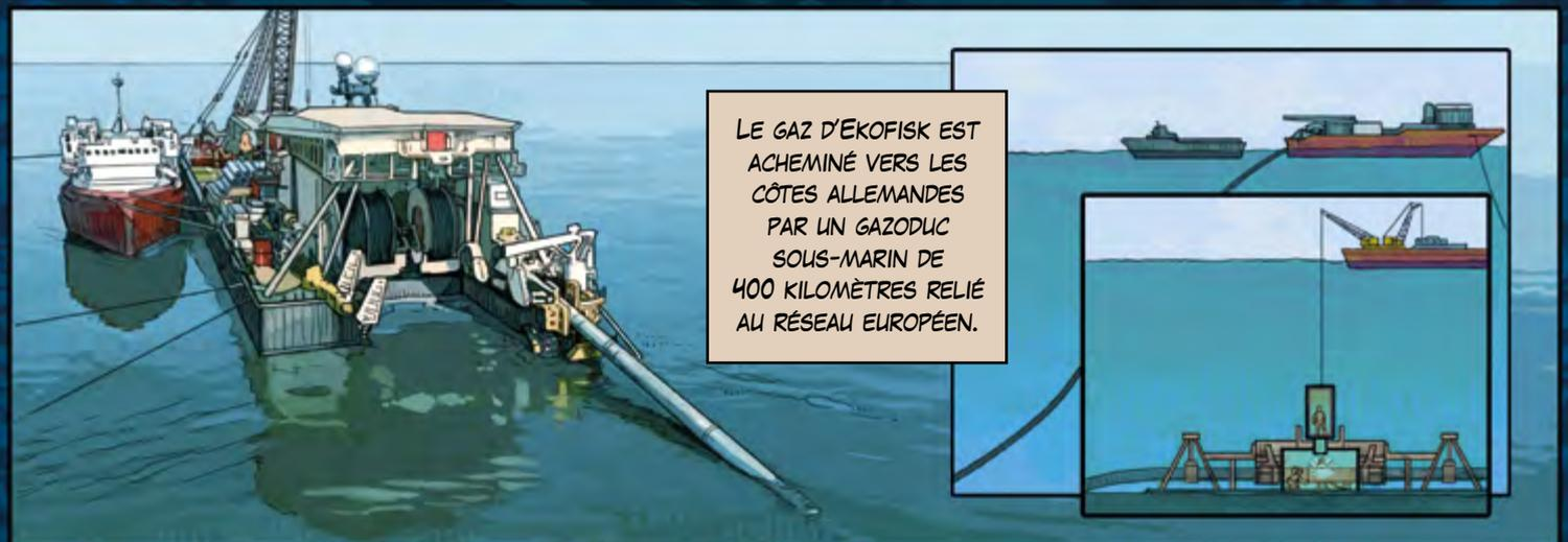
LE GAZ D'EKOFISK EST ACHÉMINÉ VERS LES CÔTES ALLEMANDES PAR UN GAZODUC SOUS-MARIN DE 400 KILOMÈTRES RELIÉ AU RÉSEAU EUROPÉEN.
